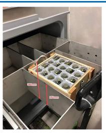
Each drawer of the DynaLOCKR F10 includes three compartments to place the explosives, six compartments in total. If an item's height exceeds the height of its compartment, blast protection to the other compartments is lost.
